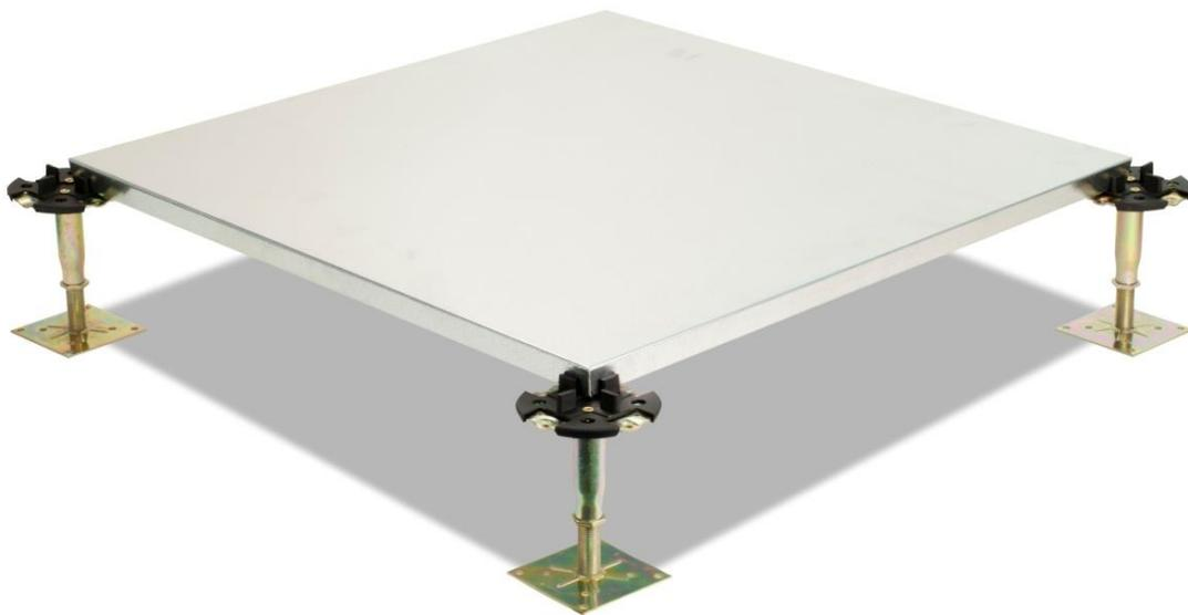
This product illustration shows the three elements: panel (particle board encapsulated in galvanised steel sheet), pedestal and pedestal cap (the black element immediately beneath the panel).
